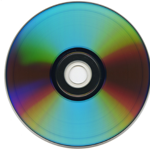
The dark ring about a half inch from the outer edge is a sure sign of bad tracks on this disk.
